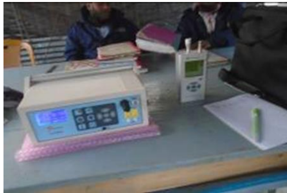
Photo 1: Respirable Dust Sampler for SPM, PM 2.5 , PM 10 and SO 2 , NO x , CO measurement instruments
